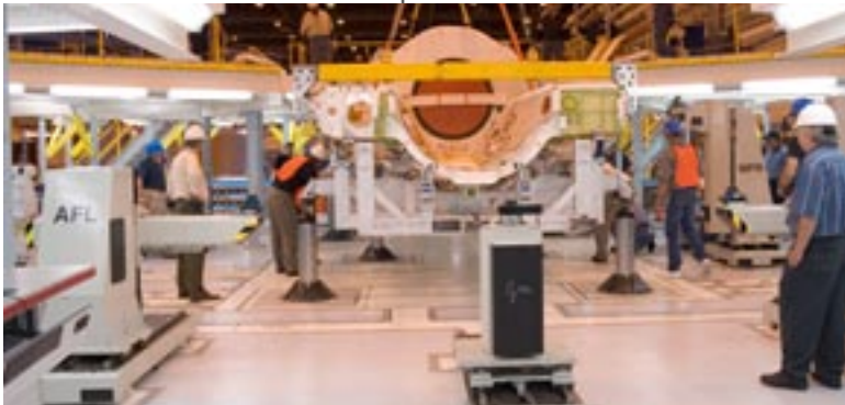
PERFECT FIT The integrated Laser Trackers in the AIT EMAS created a precise alignment for the F-35's stealth signature.
