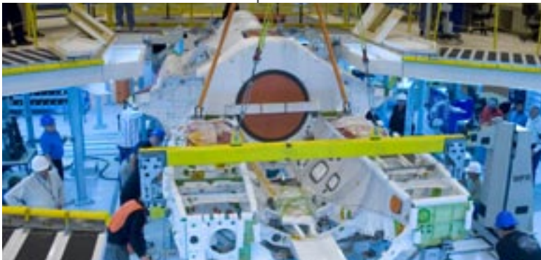
ON TARGET Laser targets on the F-35 provide data about the component's position, while positioners slide the parts together for assembly.
