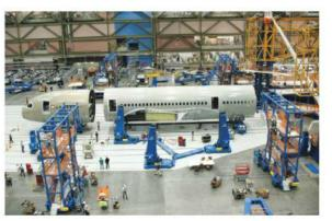
The AIT system is employed here in joining the forward fuselage to the mid-fuselage.
