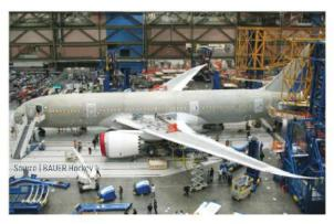
The first 787, after final assembly using the AIT positioning and joining system.
