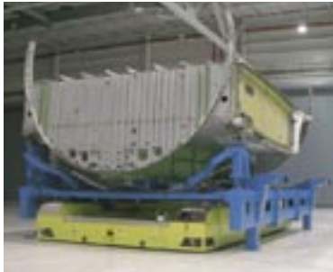
FABRICATION CART 🚚 With aft fuselage section.
