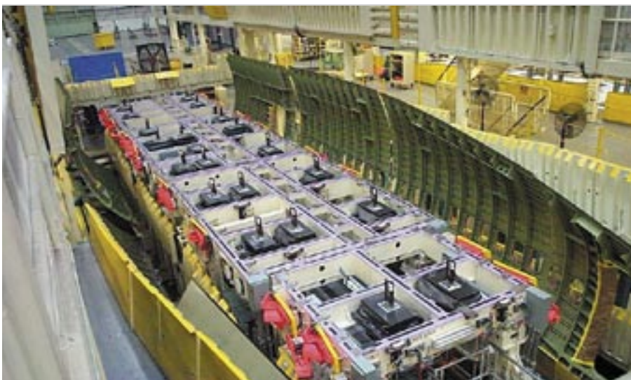
747 ASSEMBLY AIT automated the measurement and positioning of major structural subassemblies in the 747 Lower Lobes and major assembly areas.
