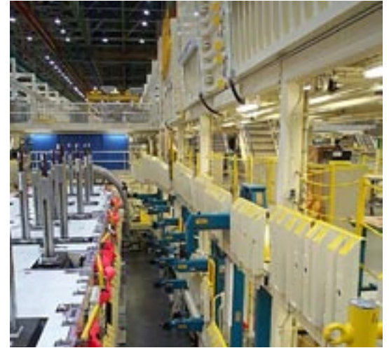
AIT INNOVATION The new Determinant Assembly simplified aircraft assembly with part-to-part indexing.
