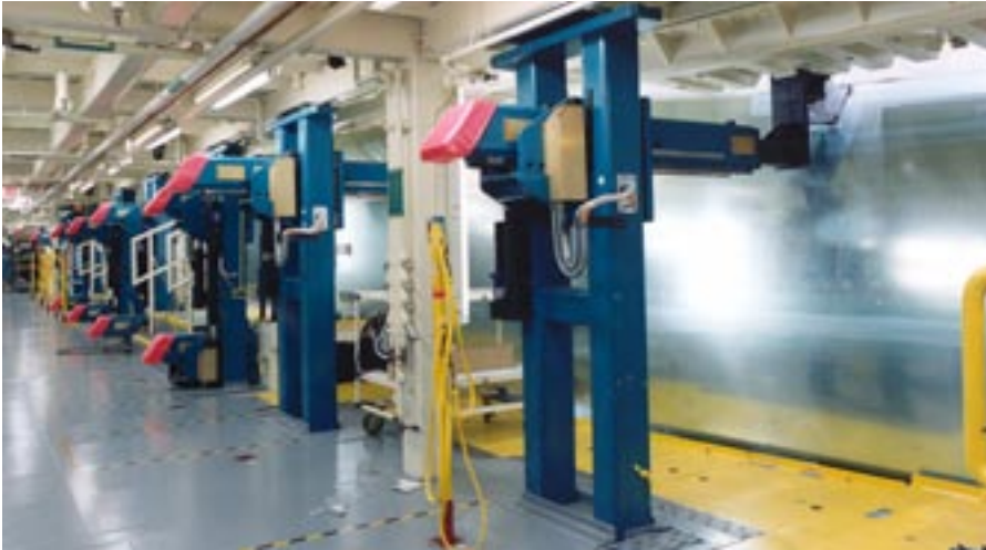
PRECISE CONTROL 13 automated fixtures with over 200 positioners and approximately 700 axes of servo motion.
