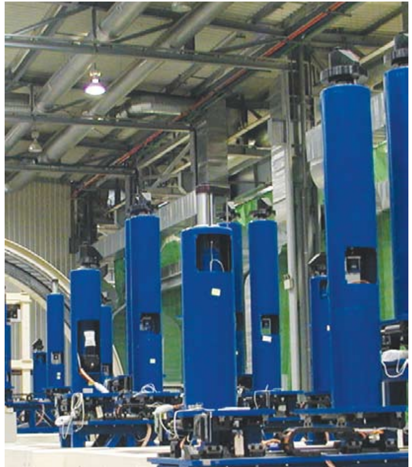
A380 SECTION 19 ⚡ Fuselage Assembly Tools for Airbus in Spain.
