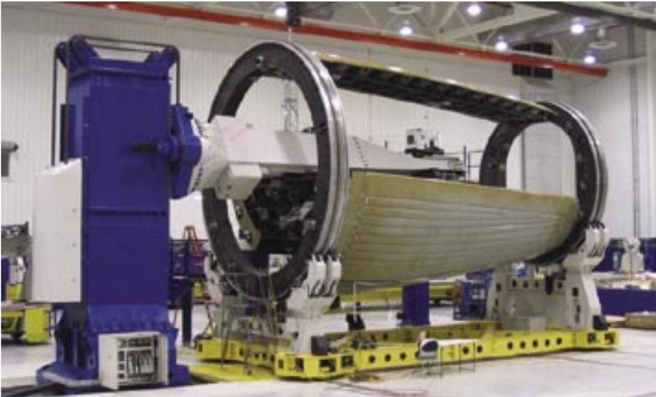
**AUTOMATED ASSEMBLY** For Vought, AIT delivered a mandrel assembly/disassembly system for the 787 Dreamliner Sections 47/48.
